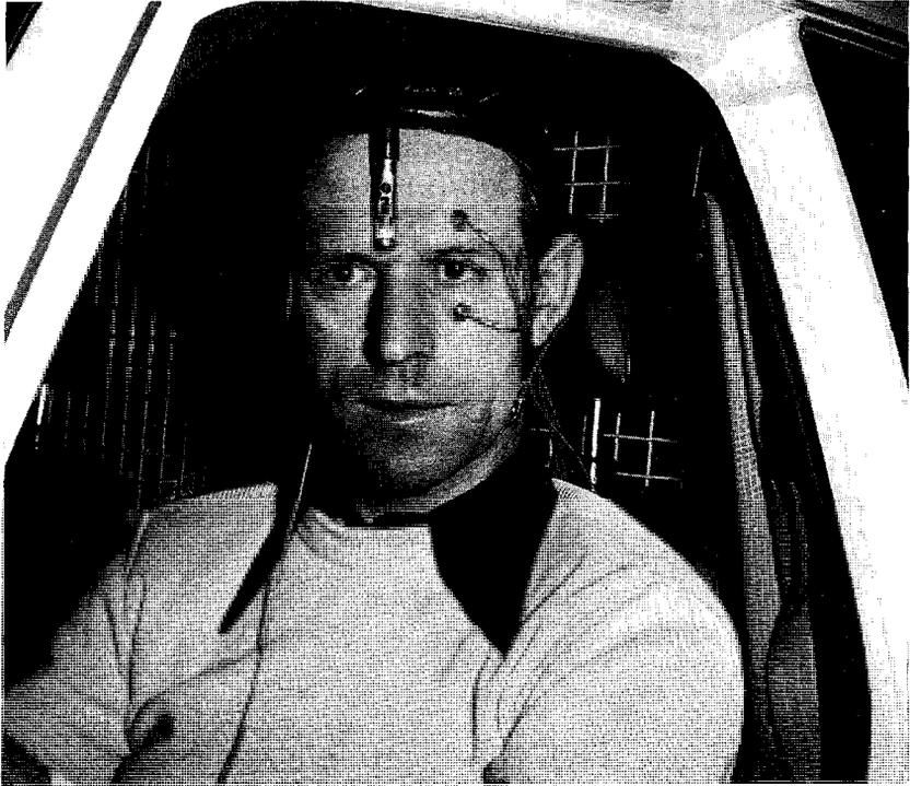
Fig. 25. Apparatus for recording gaze movements within the observed scene. From Blaauw.
