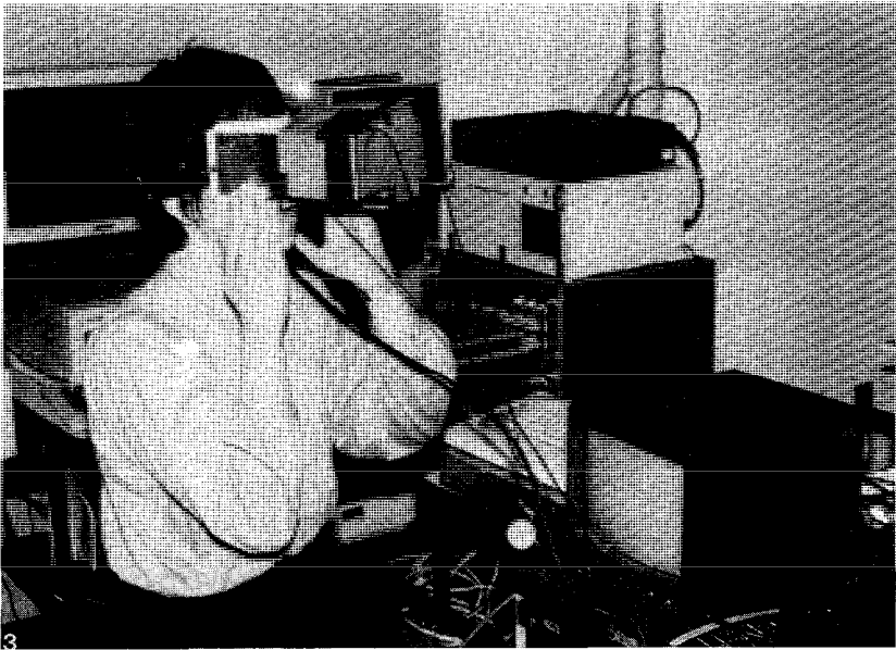
Fig 3 The Eye Mark Recorder and the liquid crystal display are mounted on a headset unit
