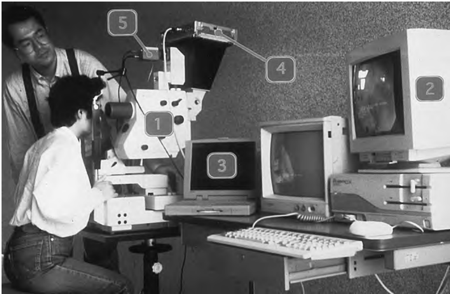
Fig. 1. The system for a new fundus perimetry. 1. Infrared fundus camera; 2. pursuit device; 3. target device; 4. CCD camera; 5. color liquid crystal monitor.
